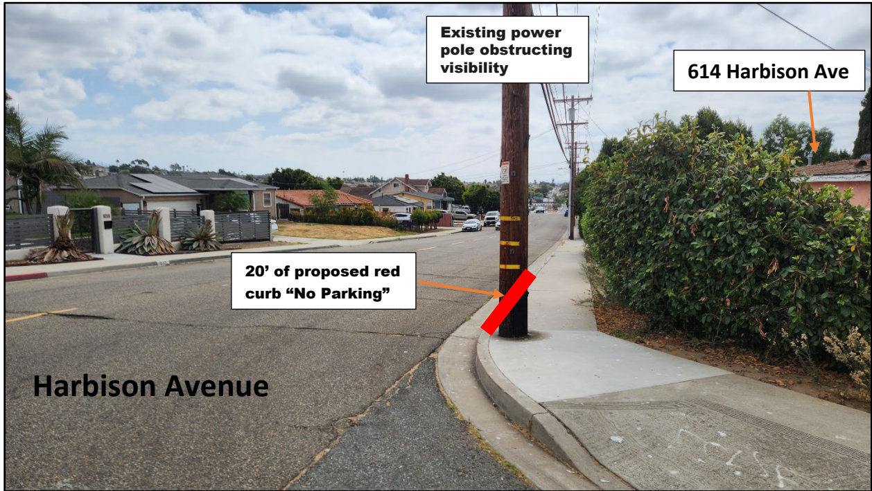
Location of proposed red curb "No Parking" on the south side of E. 6 th St, west of Harbison Ave (looking west)
