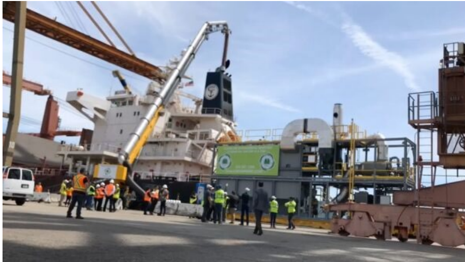
The Shorekat system, part of the Pasha Green Omni Terminal project. The system was unsuccessful, and Pasha intends to replace it. Photo courtesy of Clean Air Engineering - Maritime Inc.
