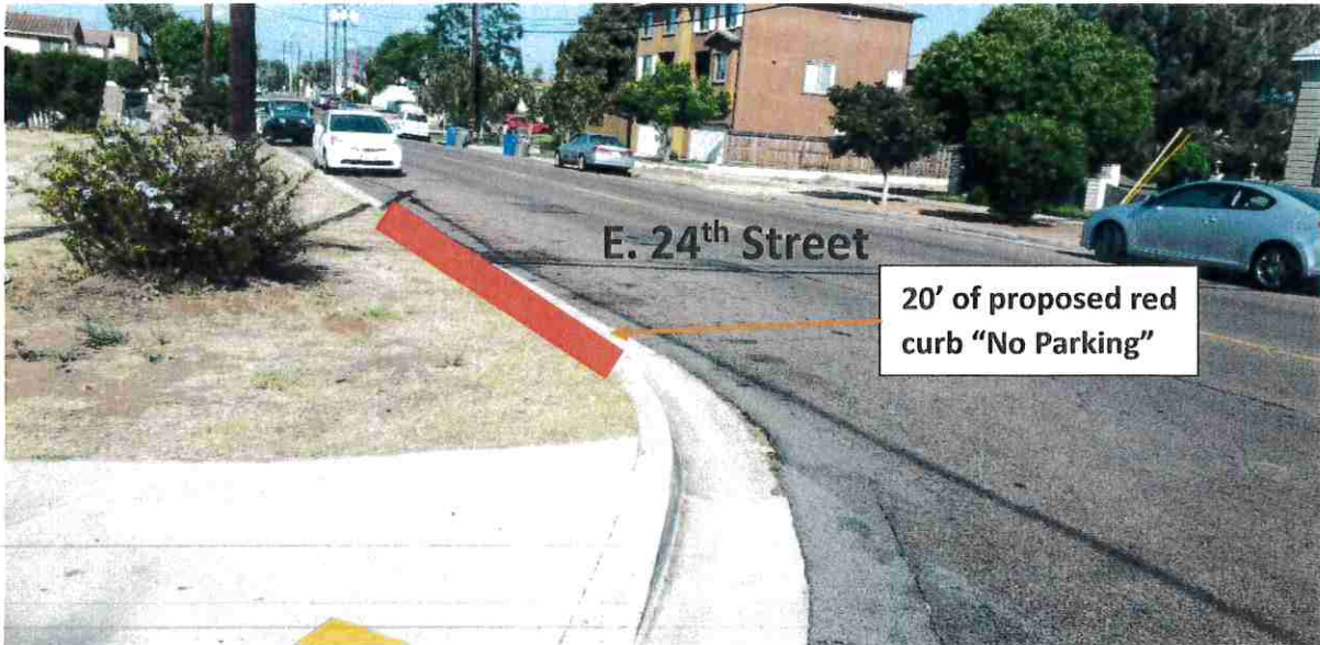
Location of proposed red curb "No Parking" on E. 24th Street (looking west)
