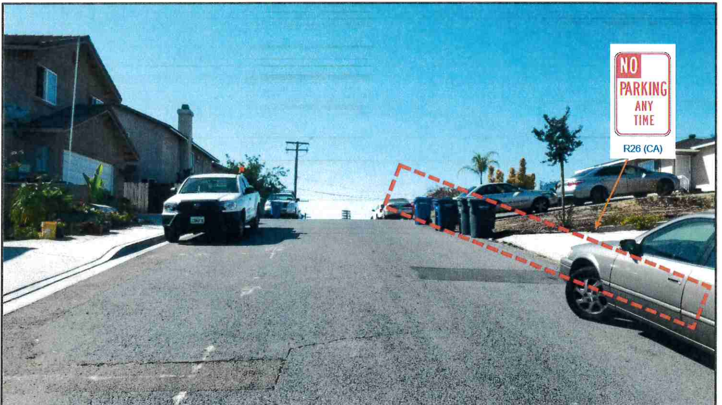
Proposed installation of 230' of "No Parking" signage on the east side of 400-500 block of T Ave (looking north)
