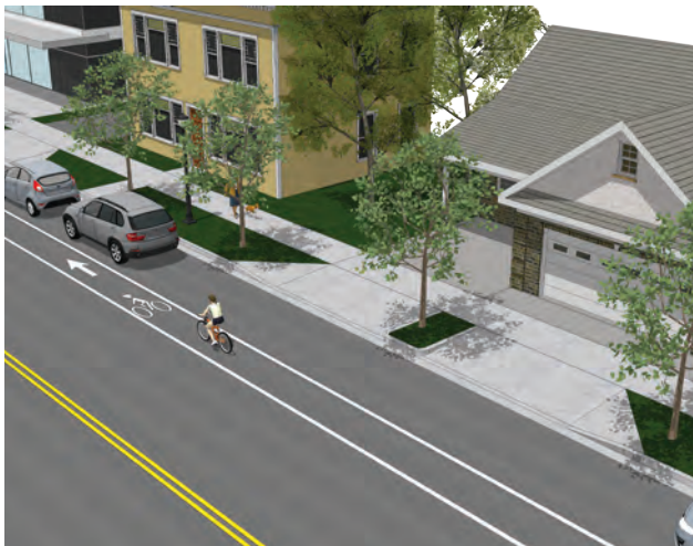
Tree planter island bisects a wide driveway providing continuous tree coverage
